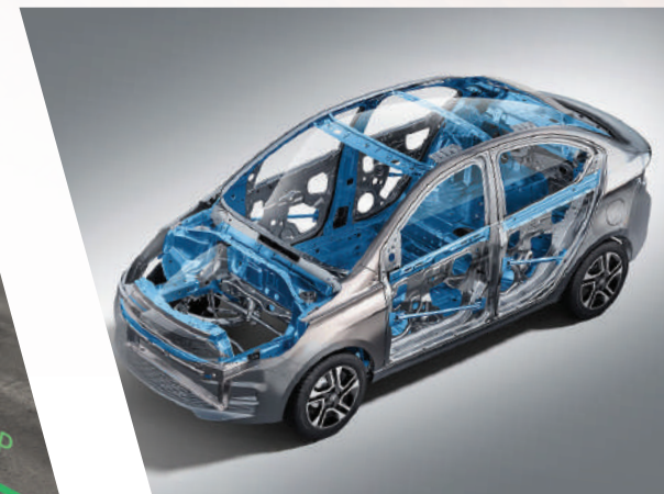
Energy-Absorbing Body Structure
