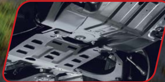
Underbody protection kit Steel skid plate and engine bottom guard to safeguard the key vehicle aggregates.
